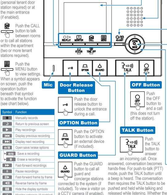
a CCTV camera (if enabled), push the GUARD button
