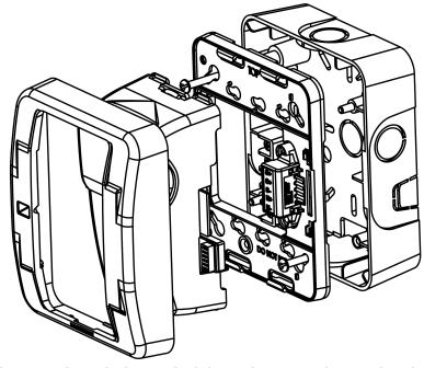
NOTICE: • GSB BACK BOX IS FOR USE WITH GEH, GES AND GEC SERIES, WALL MOUNT HORNS, STROBES AND HORN/STROBES
