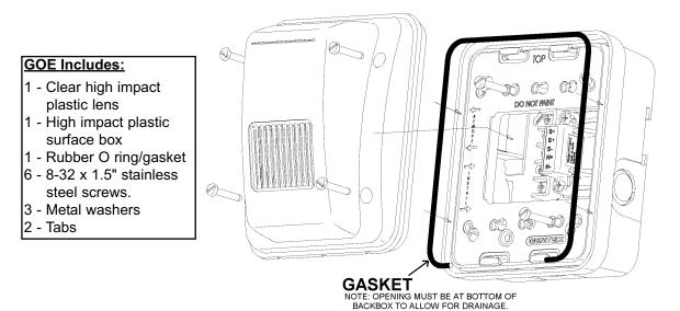
Insert gasket in between the box and mounting bracket. The signal (not shown) shall be inserted in the mounting bracket prior to attaching the cover.
