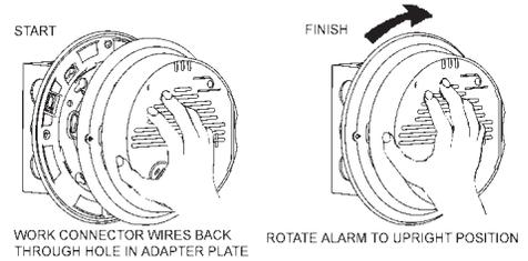
3. Place smoke alarm up to mounting plate, rotating it clockwise until smoke alarm firmly snap locks into place. Keep smoke alarm parallel to the mounting plate so tabs on plate seat correctly into the smoke alarm.
