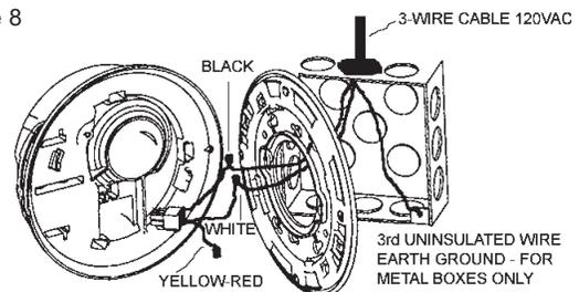
**NOTE/YELLOW-RED WIRE:** The yellow-red wire from the smoke alarm is for tandem connection only. DO NOT USE, AND DO NOT REMOVE INSULATION CAP UNLESS CONNECTING ANOTHER SMOKE ALARM.
