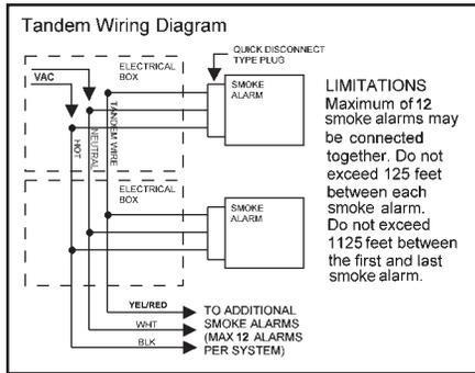
1. Run a minimum of 16 gauge, 3-conductor cable, plus ground (4 wires) to the first junction box from a power supply and between all smoke alarms that are to be connected together. Use UL listed Class 1 wire.
