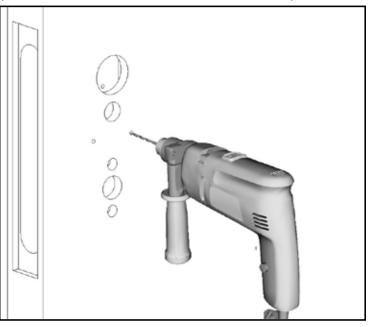
**NOTE:** When installing, make sure lock is unlocked, deadbolt is retracted and indicator shows green window (unsecure / vacant)
