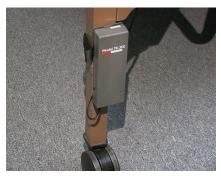
The TR-300 Extended Range Transmitter has a switch on the side of the unit to turn the transmitter on for instant or delayed operation or off to allow the caregiver to work with a patient and not have the alarm sound.
