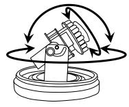
Move the camera vertically, horizontally, or rotate the lens to change the lens angle.
