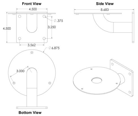
ETP-MBKT fits a 4" square box or a 1900 box and extends 8.75" from a wall. Tube is hollow to enable wires to run from ETP-EL into a conduit box.
