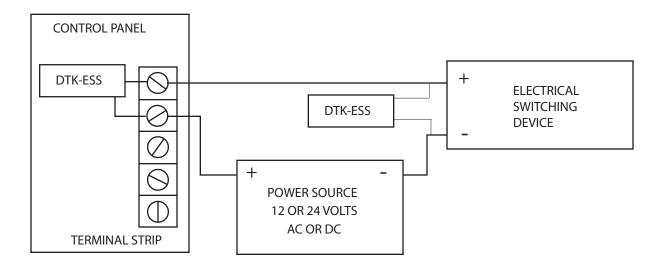
Each electrical switching device will require 1- suppressor to be installed across the relay contacts located at the control panel, and the 2nd suppressor to be installed across the leads of the switching device solenoid. The DTK-ESS is a bipolar device and can be installed without regard to polarity.
