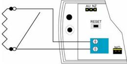
Figure 3 Wired for N/O operation
