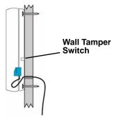
Figure 5 Mount the Transmitter to the Wall
