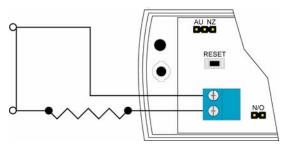
Figure 4 Wired for N/C operation
