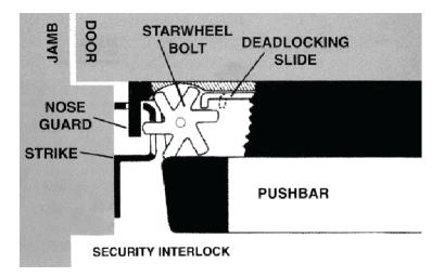
When the push bar is depressed, an interior deadlocking slide is pulled back to release the "starwheel" bolt allowing the door to open. Upon closing, the device engages the strike and the deadlocking slide returns to secure the door. Exterior entrance can be gained by key or with extensive line of entry trim available from Adams Rite.
