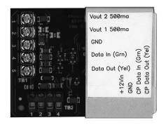
The ECP Isolator is designed to isolate burglary devices from fire devices on the ECP bus, so that a trouble on the burglary side of the bus will not affect the operation of fire devices. It can also be used in any system to prevent wire shorts or grounds from interfering with operation on another wired branch on the bus.
