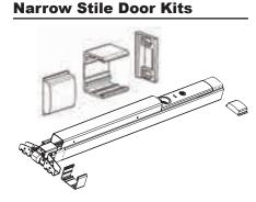
NSK - Narrow Stile Door Kit converts standard Value Series panic device into narrow stile panic device. Required when Value Series exit devices are applied to 36" and 48" glass doors with minimum 2" stiles.
