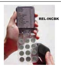
Incidents may be recorded using the Reliant Incident Book. Incidents are pre-defined and assigned numeric codes in the Reliant PLUS software. Incidents observed by the officer are recorded during a tour by entering the incident's code, using the touchmemory keypad.
