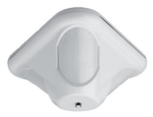
The ceiling mount DS939 PIR Detector provides a 21 m (70 ft) panoramic coverage pattern and can be used on ceilings as high as 7.6 m (25 ft). With three separate PIR sections that are fully adjustable, the DS939 provides coverage integrity at all mounting heights, plus the ability to customize the coverage for specific areas. The DS939 uses several patented processing techniques to provide excellent catch performance with freedom from false alarms.
