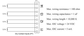
Note: All contact inputs are fully supervised. Ground fault protection impedance is 0 ohms.
