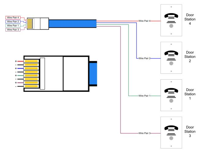
\*Note: Door Station 1 has 1 ring per cycle, Door Station 2 has 2 rings per cycle, Door Station 3 has 3 rings per cycle, and Door Station 4 has 4 rings per cycle. There is a total of 5 ring cycles.
