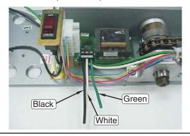
Step 5. Use the three tap connectors (provided) to splice power supply leads into units 120VAC power.
