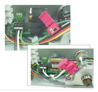
**Step 6.** Mount 433MHz Receiver to unit as shown using Velcro strip provided
