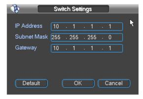
You can configure the networking settings for the internal PoE switch.
