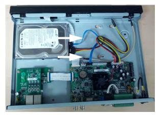
4. Turn the unit over and loosen the hard drive screws. **Do not remove the hard drive screws.**
