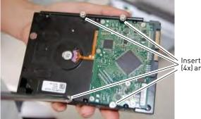
Insert hard drive screws (4x) and tighten half way
