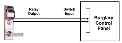
**Alarm Panel with Switched Input for Disarming**
