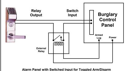
1. Group 1 Disarms a Burglary Control Panel will always disarm an alarm system. Arming should be performed by other means (such as Alarm Panel Keypad/Schedule).
