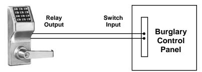
**Alarm Panel with Switched Input for Disarming**
