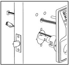
FIG. 9: INSTALL PRIMARY SIDE AND LOCK BODY (Lever, Housing & Lock body)
