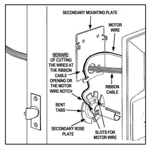
INSTALL SECONDARY SIDE LOCK BODY
