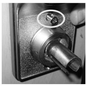
FIG. 16: SECURE THE SECONDARY TO THE PRIMARY HOUSING
