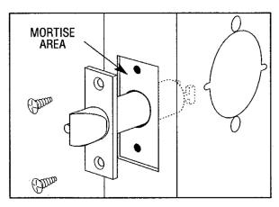
FIG. 3: LATCH INSTALLATION
