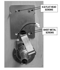
FIG. 13: SECONDARY MOUNTING PLATE INSTALLATION
