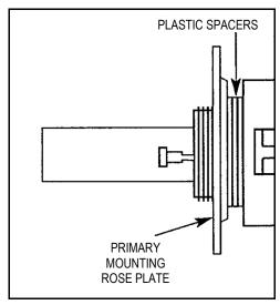
FIG. 7: ADJUST DOOR THICKNESS
