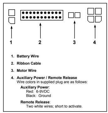
FIG. 22: WIRE CONNECTIONS
