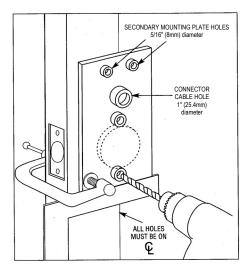
FIG. 2: ALARM LOCK INSTALLATION JIG
