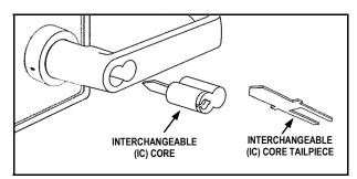
FIG. 20: INSTALL INTERCHANGEABLE (IC) CORE
