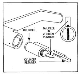
FIG. 18: STANDARD CYLINDER-LEVER, TAILPIECE AND RETAINER.
