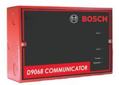
The D9068 Fire Communicator is a complete digital alarm communicator transmitter (DACT) for use with compatible fire alarm control panels (FACPs). Use dry contacts or open collector outputs for alarms and communications with the
