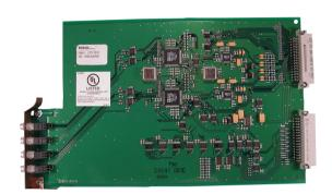
Line card with digital signal processor (DSP) technology. Answers and decodes signals from up to four telephone lines simultaneously. The Conettix D6600 Communications Receiver/Gateway will accept up to eight telephone line cards to create a total of 32 telephone lines. Needs one Connetix D6645 Telephone Line Terminator Card.
