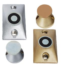
The D370 electromagnetic door holders are rugged die-cast devices for holding doors. They allow control of doorways in alarm conditions. Typical applications are in stairways or other exit pathways where it is desirable to restrict airflow yet allow free emergency access.
