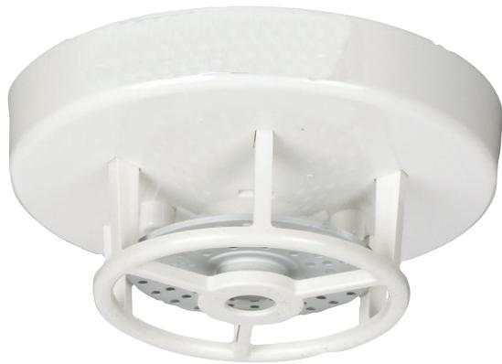
Use the D254 and D255 Fixed Temperature Heat Detectors for indoor confined areas where a fire increases air temperature slowly and where there is a substantial increase in air temperature before the fire breaks confinement. Furnace rooms, closets, bathrooms, and other confined areas are appropriate applications for fixed temperature detectors.
