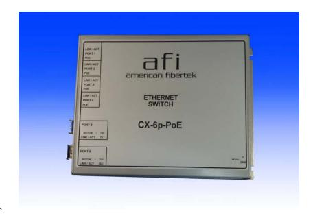
The American Fibertek CX-6p-PoE Series transmits and receives (4) copper 10/100 Base-TX Ethernet signals at the RJ45 ports and (2) 1000 Base-X over copper or fiber using SFP ports.
