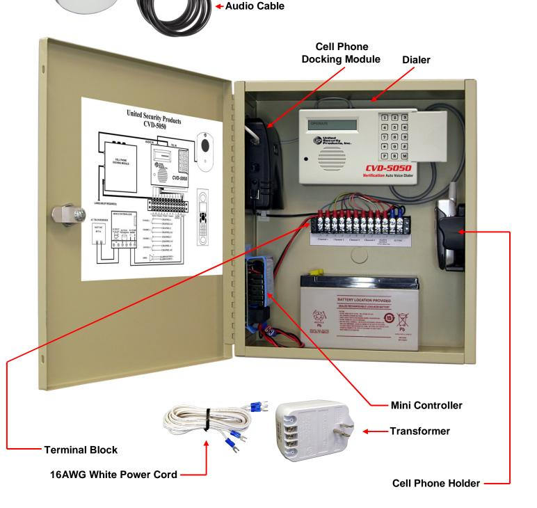
Cell Phone included with CVD-5050P and CVD-5050PS Battery not included with Systems
