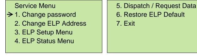
To change the CV-TAC400 DIP Address, enter the new address using the number keys. Select an address from the table below. To save the address you have just entered press the # key. To exit without changing the password enter the \* key.
