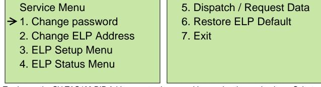
To change the CV-TAC400 DIP Address, enter the new address using the number keys. Select an address from the table below. To save the address you have just entered, press the # key. To exit without changing the password enter the \* key.
