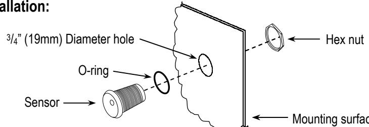
**Note:** To ensure proper operation, make sure no objects sit or come within 11 3/4" (30cm) (60° to the left and right) of the front of the IR proximity sensor to avoid interference.
