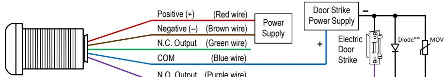
\*\* Suggest connecting a diode and metal oxide varistor (not included) as close as possible and in parallel with the controlled output device. This absorbs possible electromagnetic interference to prevent damaging the IR proximity sensor.
