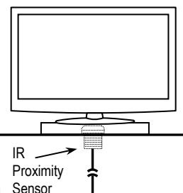
Place the sensor under a painting or other valuable object. If the object is removed from the sensor, the sensor will trigger an alarm to alert the owner that the item is out of place.
