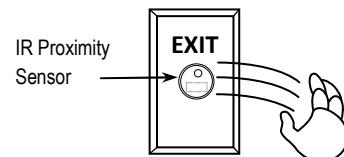
Mount the sensor to a wall or plate in a protected area. A user can wave his or her hand in front of the sensor to unlock an electronic door lock, allowing sanitary, protected egress.
