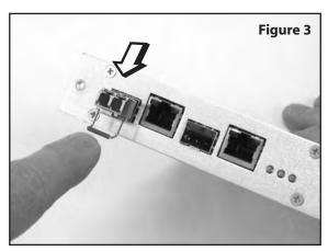
To remove an SFP sub-module from a connector cage, perform the following steps:
