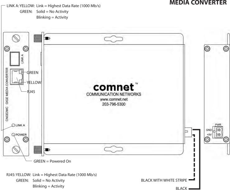
**WARNING:** Unit is to be used with a Listed Class 2 or LPS power supply rated 9-12 VDC @ 1A. **WARNING:** This unit should be installed in a restricted access location; available through the use of a lock and key or other means of security. Access should be limited to service personnel who have been instructed about the reasons for the restrictions to the location. Any and all precautions should be taken and controlled by the authority responsible for the location.
