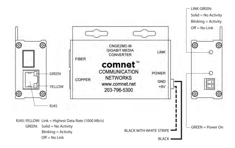
WARNING: Unit is to be used with a Listed Class 2 or LPS power supply rated 9-12 VDC @ 1A.
