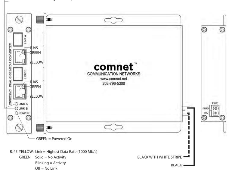
WARNING: Unit is to be used with a Listed Class 2 or LPS power supply rated 9-12 VDC @ 1A.
