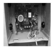
6. Grab the hexagonal spacer in the top left corner and twist to the side so that the spacer breaks off.
