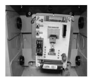
18. Slide the detector down so that the screws bottom out in the silver adaptor plate slots. Tighten the 2 screws.
