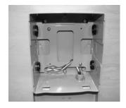
14. Remove the screw holding the top housing onto the new detector and discard the screw and top housing.
