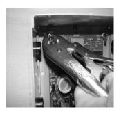
7. Break off the spacer on the upper right hand side of the box. Then break off the long hexagonal spacers on the bottom left and right corners.
