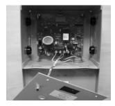
4. Loosen the screws holding the power and interconnection wires. Make a note of which colored wire goes to which connection.
