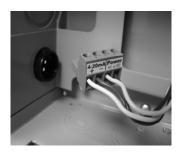
16. Install the connections in the back of the detector. If a fan or alarm is being controlled by the detector, the appropriate wires should be connected before installing the connector.
