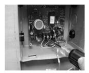
5. Remove the wires from the printed circuit assembly so that they are free.
