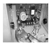
The printed circuit assembly will now be loose in the grey metal box. Remove the printed circuit assembly.
