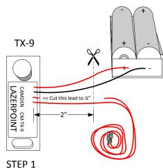
Cut the middle red lead to ¼" as it is not used. Cut both battery leads, and the remaining switch lead to approximately 2" long. Strip the insulation back on the 3 long ends to approximately ¼".
