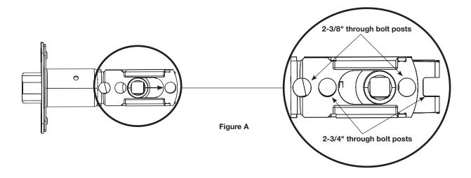
**NOTE**: The latch can be installed in only one of two ways - with the *bevel* (slope) of the latch facing out or facing in **while standing outside of the door.**
