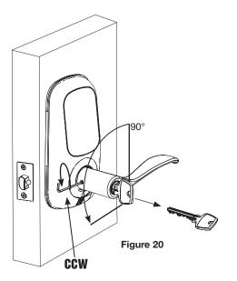
17. Rotate thumbturn counter-clockwise to horizontal position (Fig. 21).
