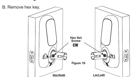
13. Install cylinder in exterior lever.
