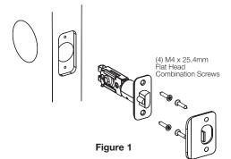
2. Install strike on the door frame, using two (2) M4 x 25.4mm screws supplied, making sure to allow for the latch to be **centered** in the strike.
