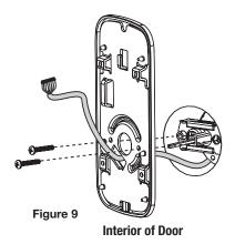
7. Secure both assemblies by inserting (2) M4 x 25.4mm pan head machine screws through the mounting plate and into the slightly extended **through posts** of the exterior escutcheon (Fig. 10).
