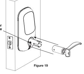
15. Secure lever handle by inserting hex key and rotating set screw **CCW** (Fig. 20).
