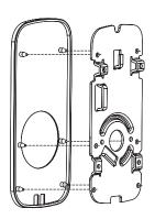
5. Remove the battery cover from the back of the interior escutcheon (Fig. 8) by loosening the captive Phillips head screw, then lifting the cover up and out. Note tabs at bottom of cover.
