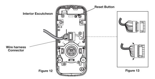
10. Install and secure interior escutcheon to interior mounting plate using (4) M4 x 8mm pan head machine screws through the interior escutcheon into the mounting plate (see Fig. 14).
