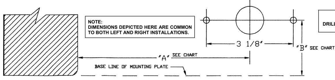
DRILL 1" HOLE THRU DOOR FOR PULL.
