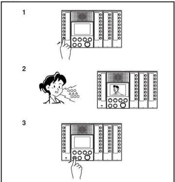
Calling a master station from a master station and communicating
