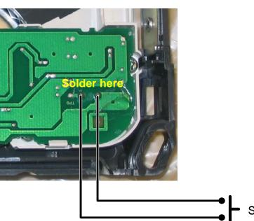
3) Solder two wires to back of switch as indicated by diagram.
