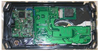
1) Remove front cover of AX-DV by removing security screw on bottom of unit.
