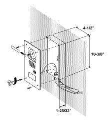
**AX-DVF-P:** Provide a wall surface opening for roughin backbox (supplied), using dimensions shown. Note: If surface mount is required, use the Aiphone SBX-DVF-P (sold separately).
