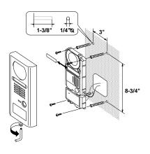
**AX-DV-P:** Provide mounting box or wall opening sufficient for both the CAT-5e cable (from the AX CEU) and the HID card reader wire pigtail.
