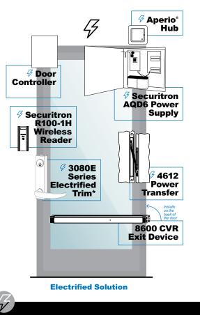
**Electrify the door with a 3080:** The 3080 Series Electrified Entry Trim provides simple access control right in the lever set. It enables remote activation of the locking function without unlatching the door, making this trim ideal for stairwell and fire doors.
