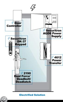
**Electrify the door with a 2190:** The Dual Force 2190 combines the access control capabilities of a latch with the security of a deadbolt. Provides free egress out for safe passageway and can be easily integrated into an access control system.
