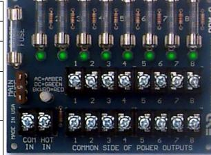
Input Voltage ..... 10.5 to 12.4vdc or 22.7 to 25.2vdc Output Voltage ..... virtually the same as Input Current, Typical, with No Output Load ...... 90-160mA Outputs 1–8 continuous duty each ..... 1.23 Amps Voltage Trigger ...... 20% < Input min. 30vdc max. Voltage Trigger isolation ..... Optical EOL (End of Line) Trigger ..... Trip +-50% of 2.2K Ω Transfer Relay Contacts ...... 15Amps Trouble Form C Contacts ...... 2A 120vac/1A 220vac Triggered Form C Contacts ...... 2A 120vac/1A 220vac
