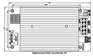
or both 12vdc and 24vdc at the same time. When outputs 1 & 2 are connected in parallel, the output is 13.75vdc at 20 Amps. When outputs 1 & 2 are connected in series, the output is 27.5vdc at 10 Amps. Because each output is independently regulated, you may draw additional current from the 12V output 1, while using the 24vdc output at the same time. The 12v current used has to be subtracted from the 10
