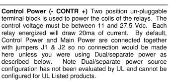
Main Power (- POWER +) Two position un-pluggable terminal block provides the power to the outputs to be distributed and power to Control through J1 & J2. In a normal application the Power must be between 11 and 27.5 Vdc and would be connected here.
