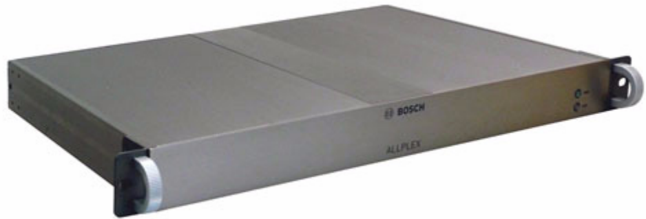
Figure 4.1 Rackmount brackets and handles installed on the panel
