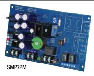
SMP7PM supervised power supply/charger converts a low voltage AC input into a 12VDC or 24VDC output. This unit has a wide range of applications for access control, security and CCTV system accessories that require additional power.
