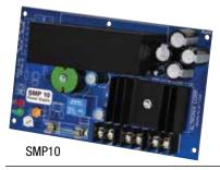
SMP10 power supply/charger converts a low voltage AC input into a 12VDC or 24VDC output. This unit has a wide range of applications for access control, security and CCTV system accessories that require additional power.
