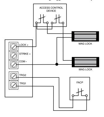
Fig. 4 - Typical mag lock with fire alarm tie-in using aux output installation:
