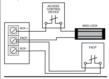
Fig. 5 - Latching fire alarm tie-in with manual reset:
