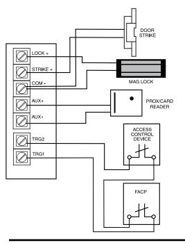
Fig. 3 - Typical dual mag lock installation with fire alarm tie-in using trigger controlled outputs:
