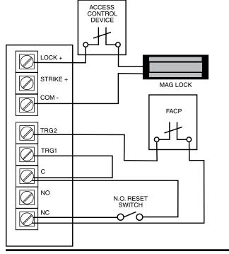
Fig. 6 - Multiple AL175UL(X) power supply connections:
