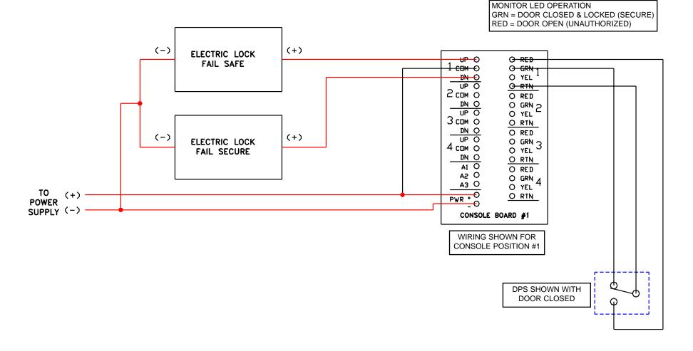
ALL POWER WIRES MUST BE 18 AWG OR LARGER. ALL SIGNAL WIRES MUST BE 20 AWG OR LARGER.
