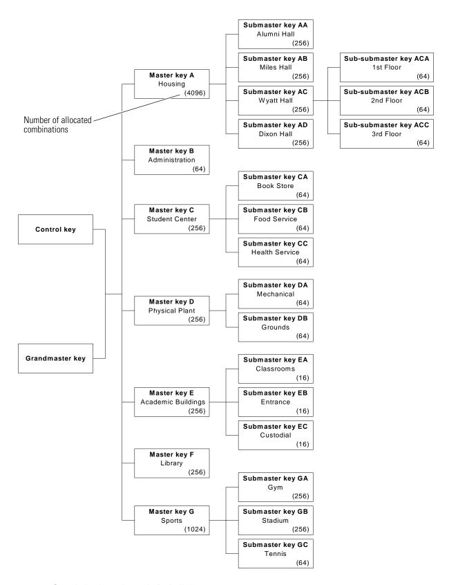
**Figure 5.2** Sample keying schematic for buildings
