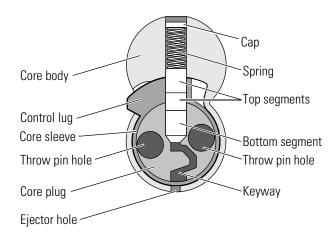
Figure 3.2 Cross-section view of core
