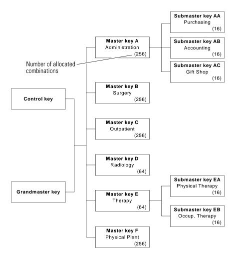
**Figure 5.3** Sample keying schematic for departments
