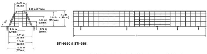
\* STI-9880 - 62.75 in. (1593mm), adjustable length reduces to 51 in.(1295mm) STI-9881 - 98.25 in. (2495mm), adjustable length reduces to 74.75
