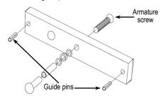
**Tip:** Use a thread-locking compound on the armature screws to ensure a long-lasting installation.
