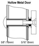
Drill two 5/16" (8mm) dia. holes through the armature-plate side of the doors for the armature screws. Then drill two 5/8" (16mm) dia. holes for sexnut screws on the opposite side of the doors.
