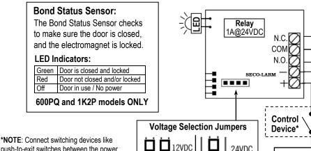
push-to-exit switches between the power source and the positive terminal on the lock. Connecting switching devices to the negative terminal may cause a delay in unlocking.
