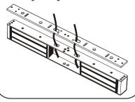
13. Push the electromagnet against the mounting plate so the ends are flush with the each other. Use the Allen wrench to screw the hex-head mounting screws through the bottom of the electromagnets into the mounting plate.
