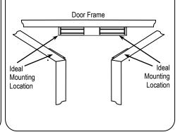
3. Place the template against the door and frame. Mark where the holes are to be drilled.
