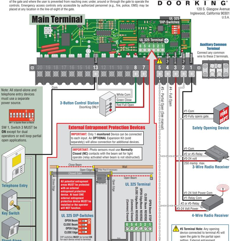
setting. External entrapment protection devices will also open the gate to the partial open setting. If the Inherent Reverse Sensor gets activated during the close cycle, it will always fully open the gate.
