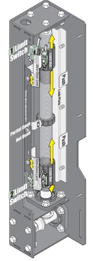
With power OFF, push and hold the lock plate down where shown to adjust the Open and Close limit nuts. After adjusting the limit-nuts, be sure that the lock-plate is engaged in the slots on the limit-nuts to prevent them from rotating.
