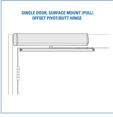
The 9130 BENCHMARK by LCN is an electrically powered low-energy operator. It provides easy access for people with disabilities, the elderly or the frail. Designed primarily for automatic opening applications that occasionally require manual opening. The BENCHMARK is a cost-effective solution for retrofitting an activated or manual door.
