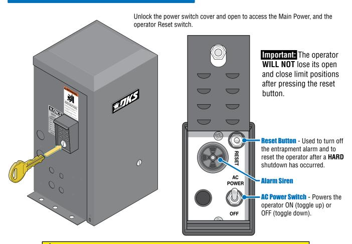
Every time the 9100 is powered up, the First open command will automatically run "Multiple gate cycles" that will locate and remember the gate's open and close positions (See page 22).
