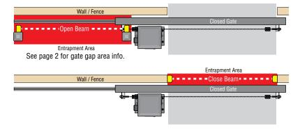
OPEN Edge/Beam Reverse: Obstructed reversing edge or photo beam will reverse the gate to the close position during the opening-direction only.
