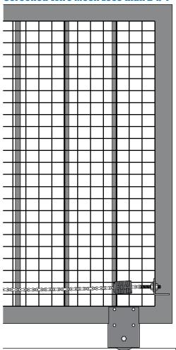
DoorKing recommends installing screened wire mesh on the **ENTIRE** gate **AND** and on that portion of the adjacent fence that the gate covers in the open position. (See above).
