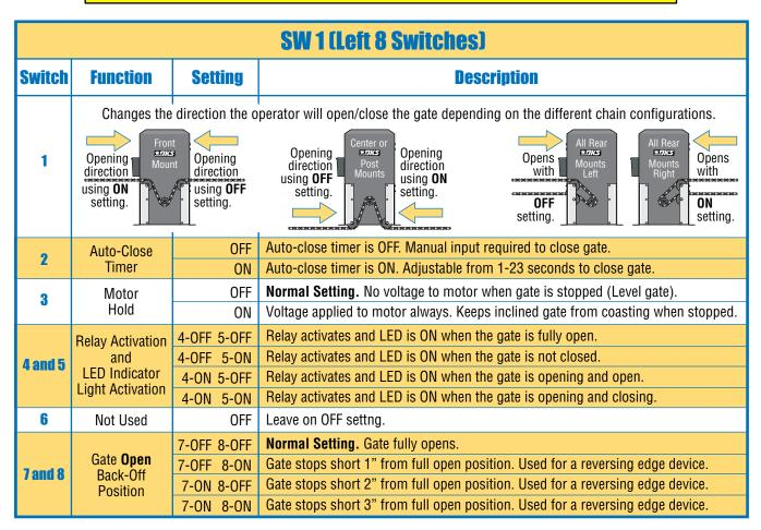
SW1Switch 1 Must OPEN the gate upon initial AC power up and open command. If the first open command begins to close the gate, turn AC power off and reverse this switch. Opening direction will vary depending on the type of installation (See above).
