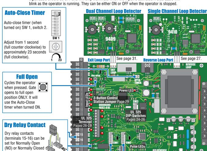
(NC) operation by placing the relay shorting bar on the N.O. or N.C. pins respectively. SW 1. switches 4 and 5 must be set to control relay. See
