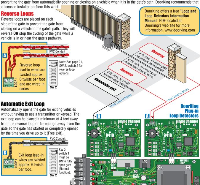
Note: The plug-in exit loop detector can be wired to partially open gate 14-Ft. if SW 2, switch 1 is turned **OFF**. A jumper wire must be connected from terminal #10 to terminal #5 (See next page for more information).
