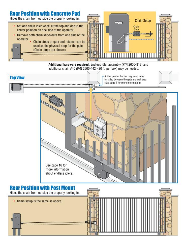
Additional hardware required. Post base plate (P/N 2600-418) 4 x 4 steel posts not available from DoorKing.
