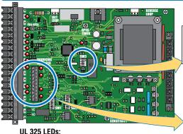
LED ON: Connected device has been activated. LED remains off during normal operation.
