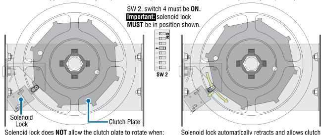
Solenoid lock does **NOT** allow the clutch plate to rotate when:
