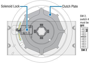
Solenoid lock does **NOT** secure the clutch plate during an AC power failure or turning AC power off. Gate can be immediately manually operated during these conditions.
