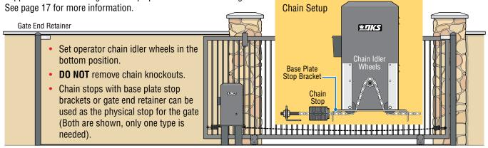
**Additional hardware required.** Post base plate (P/N 2600-418) 4 x 4 steel posts not available from DoorKing. Base plate stop brackets (P/N 2600-970) bolts on post base plate when using chain stops. Optional chain tray kit (P/N 2601-270 10 ft section) and additional chain #40 (P/N 2600-442 - 20 ft. per box) may be needed.
