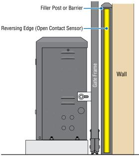
A filler post or barrier may need to be installed between the gate and wall area to reduce the distance to 2 1/4" or less. A reversing edge should be installed on the post or barrier for safety (See page 2 for more information).
