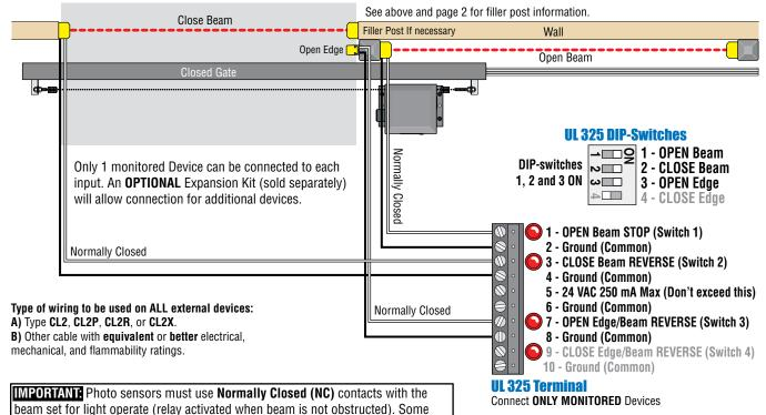
power photo sensors that can be plugged into the built-in wiring manual for more information about their specific relay function. convenience outlets located on the operator (See page 24).
