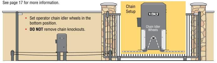
**Additional hardware required.** Post base plate (P/N 2600-418) 4 x 4 steel posts not available from DoorKing. Endless idler assembly (P/N 2600-818). Additional chain #40 (P/N 2600-442 - 20 ft. per box). Gate end retainer (P/N 1204-004).
