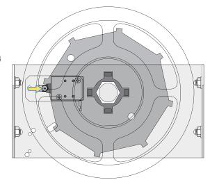
Solenoid lock **WILL** retract and secure the clutch plate during normal operation **ONLY** if operator senses an **unauthorized** manual open attempt. Gate will **NOT** be allowed to move.
