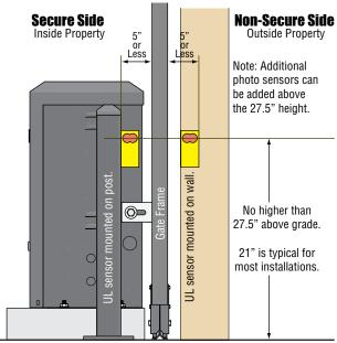
Photo sensors may be installed on either side of gate frame, as close as practical to the gate but no further away than 5".
